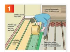
Where possible fit additional insulation beneath subfloor. If a timber subfloor this can be fitted between the joists, if concrete subfloor you can use Prowarm Backer Pro Insulation boards.
