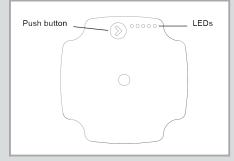
The user interface is designed with a single push button, one red/green LED and four yellow LEDs.
