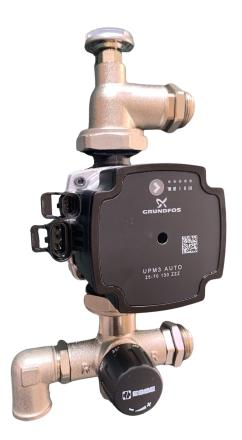
Kv: 3.4Kv (Up to 220sqm / 18kW) Temperature range: 20°C - 55°C Max temperature range: Continuously = 95°C / Temporarily = 100°C Maximum supply pressure: 10 Bar
