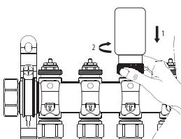
Attach the ABA to underfloor heating manifold thermostatic valves, on the return bar. When installing the THB23030 / THB2430 ensure it is fully tightened onto the manifold. Actuator is in fully open position, out of the box, for easy installation.
