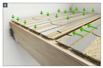
• Secure the panels together using a D4 adhesive on BOTH sides of the tongue and groove and fit together. The panels should then be glued and screwed to the joists.
