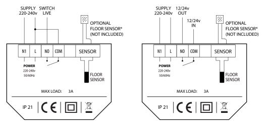
\*NB: No Polarity on floor sensor terminals
