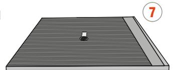
**STEP 7** Spread the adhesive evenly over the area where the shower tray is to be installed, being carefully to clean away any adhesive on the rim of the trap.
