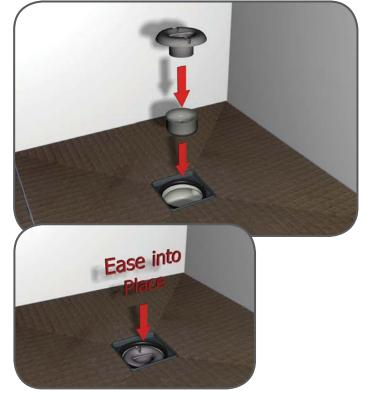
6. Ease the Shower Drain Internal Bowl into the Shower Drain. Ease the Shower Drain Internal Dome into the Shower Drain.
