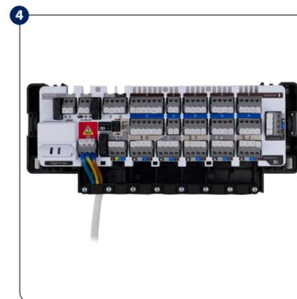
For safety use fastening strap to prevent power supply / thermostats wires from falling out.
