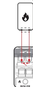
Boiler output - this is a volt free output (COM / NO) which controls heating system boiler. If any of thermostats connected to the control box sends signal for heating, BOILER output is activated after 3 minutes delay, giving permission for boiler to turn ON. If all thermostats connected to the control box stop sending signal for heating, then BOILER output is deactivated - this is the signal for boiler to turn OFF (BOILER output can work with 0min or 15min delay - please refer to chapter 4b).
