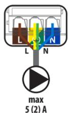
PUMP/VALVE output - this is a 230 V AC output that controls the pump and valve of the heating and cooling systems. If any of thermostats connected to the CB500 send heating / cooling signal - PUMP/VALVE output will be activated after 3 minutes. If all of the thermostats connected to the CB500 stop sending heating / cooling signal - PUMP/VALVE output will be deactivated after 3 minutes.
