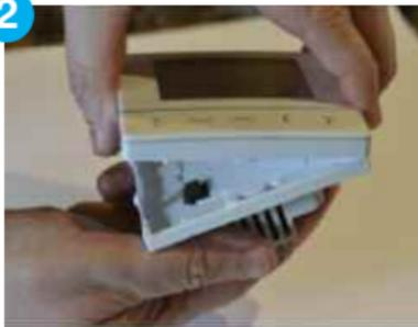
Carefully remove the front housing.
