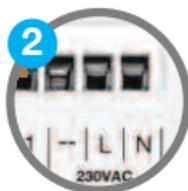
**Power Terminals 230v AC.** Used for supplying power to the unit. 230v supply can be sourced from the wiring centre or any convenient source.
