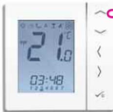
Use the up arrow to select the frost protection temperature.
