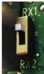
System Receiver configured to boiler receiver RX1. Refer to Boiler Receiver Instruction Manual.
