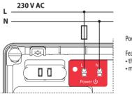
Power supply for wiring centre is 230V ~, 50Hz.
