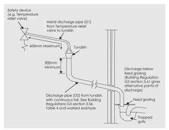
**Note:** The discharge will consist of scalding water and steam. Asphalt, roofing felt and non-metallic rainwater goods may be damaged by such discharges.
