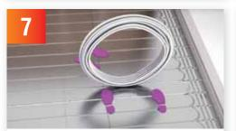
Above picture: illustration purposes only, ideally the pipe should be unrolled using a de-coiler or in the horizontal position to allow for ease of laying the pipe (This will stop the pipe trying to spring out of the boards at the end of the panels).
