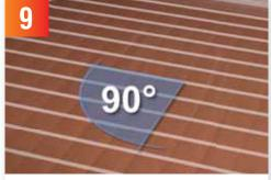
Ensure that when installing floorboards they are positioned at a 90° angle to the pipe direction.
