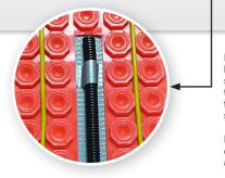
Position the floor sensor in the black conduit supplied between two runs of cable and tape into position. The sensor wire can be shortened or lengthened. If you need to cut the sensor wire you must only cut the end containing the wires. DO NOT cut the end which contains the plastic sensor.
