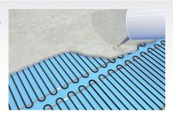
If you are using a suitable LVT/ carpet or engineered/laminate floor as the final covering then we recommend a minimum of 10mm suitable latex levelling compound to cover the heating mat/cables to ensure even heat distribution.
