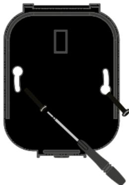
Insert fixing screws through mounting holes of the power base and tighten.
