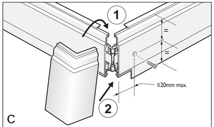
Finally, fit the corner cover in position by hooking over the top of each side of skirting, then pushing the bottom inwards until it clicks (**C**). Trim the cable cover and caulking gasket 5mm longer than required. These may then be tucked behind the corner covers and end covers to achieve a neat finish (**D**). Special external corner covers may be required in some installations. Download a template from: [www.discreteheat.co.uk/technical.html](http://www.discreteheat.co.uk/technical.html)
