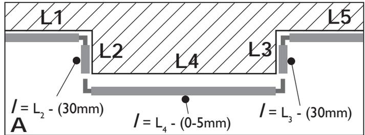
External sections of skirting are cut to within 5mm of the length of wall that it is fitting to ( $I = L - 0/5\text{mm}$ ) (**A**).
