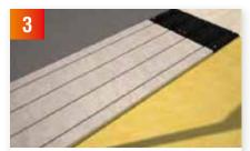
Lay the first Overlay panels against the first two End supports. Clean down the boards and ensure there is a 3mm bead of adhesive along the edges, this will ensure that the boards are secure.
