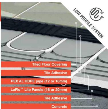
ProWarm™ LoFlo™ Lite panels utilise high compressive strength through expanded polystyrene, with a high tech aluminium foil covering. This acts as a heat conducting surface to transfer the heat from the pipes to the finished floor above.
