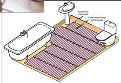
7. If required, the cable can be removed from the mesh and loops formed manually, but ensure the cables are spaced the same distance as those on the mat.
